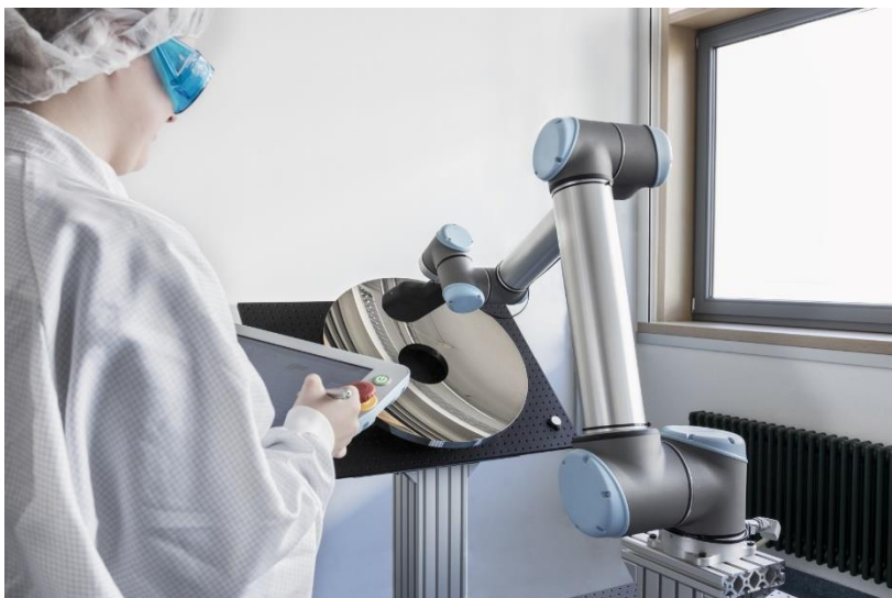
Fig. 2: Robotic Light Scattering Sensor. © Fraunhofer IOF.
